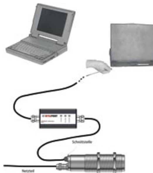
Fig.: Connection example: IKS-Ti - IP 10-USB - Laptop
