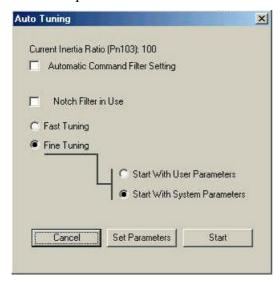
Automatic Command Filter Setting: enables the command filter function. The value of the command filter is calculated automatically and stored in parameter Pn216.
