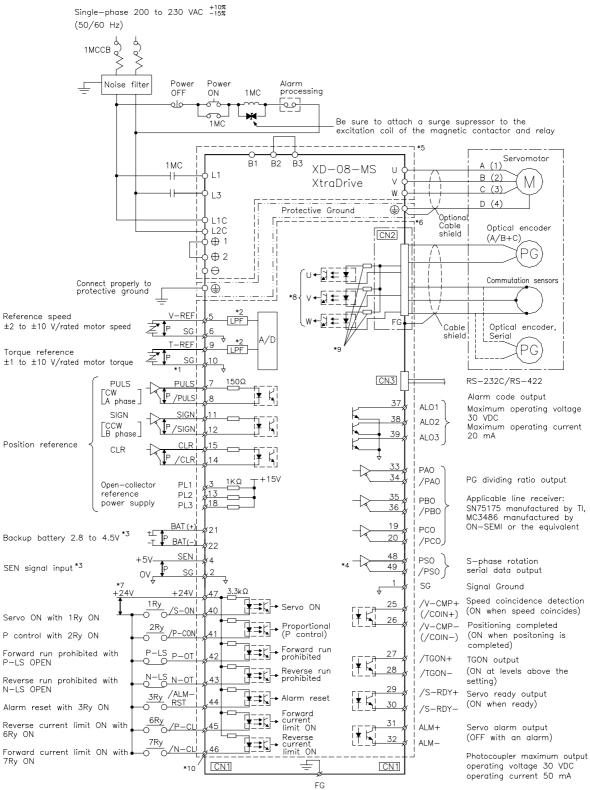
Connect shield to connector shell
