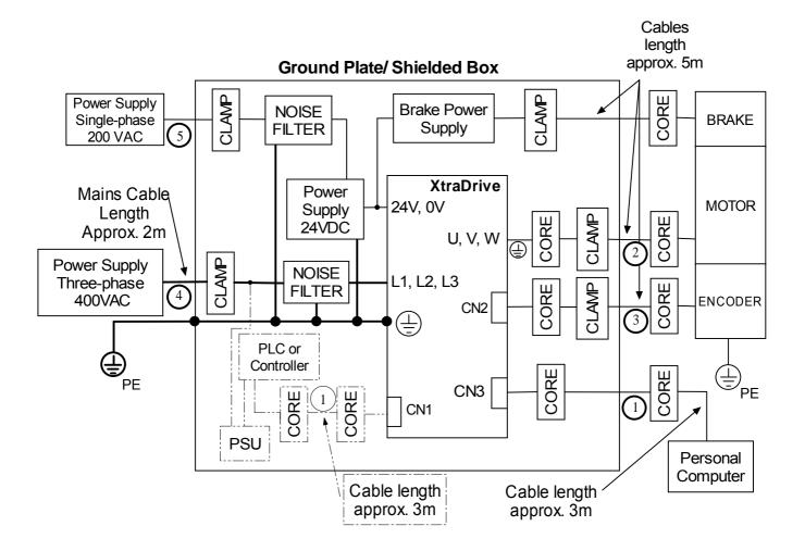
resents option with PLC or controller connected to CN1 connector.
